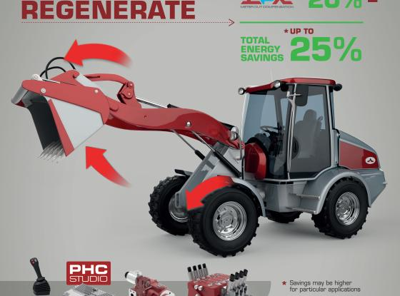
Walvoil's Adaptive Load Sensing system (ALS) can optimize and recover energy dissipated during each work phase, providing significant increase in the efficiency of machinery for agriculture, construction, and the material handling sectors. EPX (Meter out compensation) technology recovers and regenerates energy in the machine system based on the options chosen by the manufacturer. When combined, ALS and EPX, allow an overall energy saving of up to 25%.
